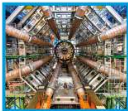
The ATLAS calorimetry system at CERN, seen here during installation, measures the energy of particles after a collision by forcing most to stop and deposit their energy in the detector.
