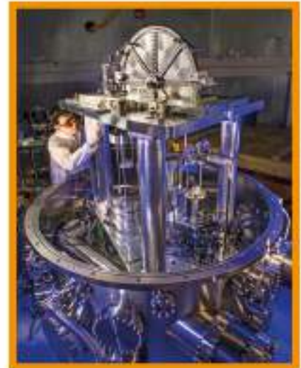
The Kibble balance at NIST produces incredibly accurate measurements, and has contributed to the recent redefinition of all base measurement units in terms of physical constants.
